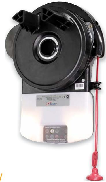
The Garador™ roller garage door opener has an ultra compact side profile that allows installation into almost any limited side-room situation. The opener features soft start/soft stop, which reduces load and wear on the opener and softens the point of contact when the door finishes closing.
