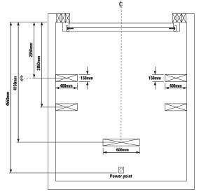
The details shown are for 3.35m Maximum height Sectional Door with Standard 330mm Headroom. Also for Intermediate Headroom of 220mm with springing to front. Measurements for motor with 2.3m C-Rail and 1m extension.
