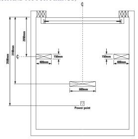
The details shown are for 2.3m Maximum height Sectional Door with Standard 330mm Headroom. Also for Intermediate Headroom of 220mm with springing to front.
