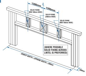
Note: The details shown are for 3.90m Maximum Height Sectional Door with Standard 330mm Headroom. Also for Intermediate Headroom of 220mm with springing to front. Measurements allow for motor with 2x C-Rail extensions.
