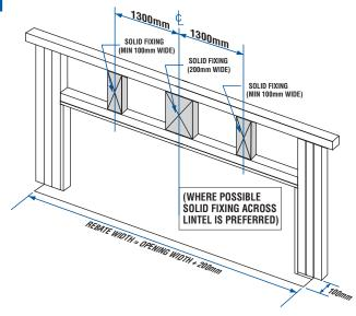
Note: The details shown are for 3.15m Maximum Height Sectional Door with Standard 330mm Headroom. Also for Intermediate Headroom of 220mm with springing to front. Measurements for doors over 2.40m high allow for motor with 1x C-Rail extension.
