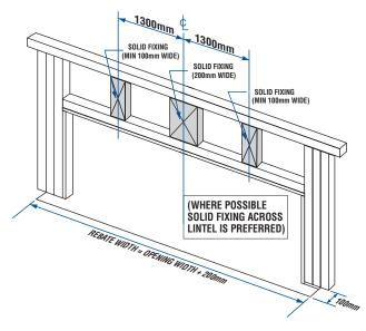
Note: The details shown are for 2.30m Maximum Height Sectional Door with Standard 330mm Headroom. Also for Intermediate Headroom of 220mm with springing to front.
