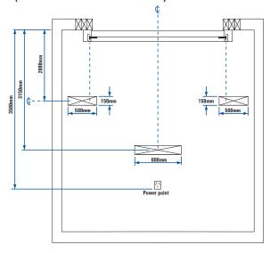
Note: The details shown are for 2.3m Maximum height Sectional Door with Standard 330mm Headroom. Also for Intermediate Headroom of 220mm with springing to front.
