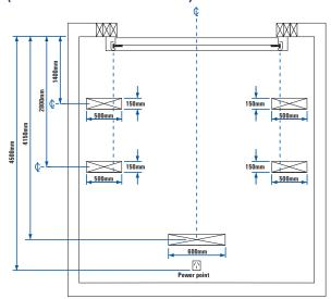
Note: The details shown are for 3.35m Maximum height Sectional Door with Standard 330mm Headroom. Also for Intermediate Headroom of 220mm with springing to front. Measurements for motor with 1m extension.
